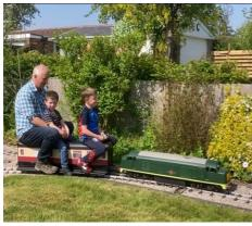
Steam locomotives use real coalfired steam. Diesel models use car batteries with electric wheelchair motors which are more accessible and affordable. You only need one loco and coach or so I tell my wife, so it is not a more expensive than a large indoor model railway. I am building wagon kits and I would like a radio controlled model that I can set running around the track while I mow the lawn. You can build them
